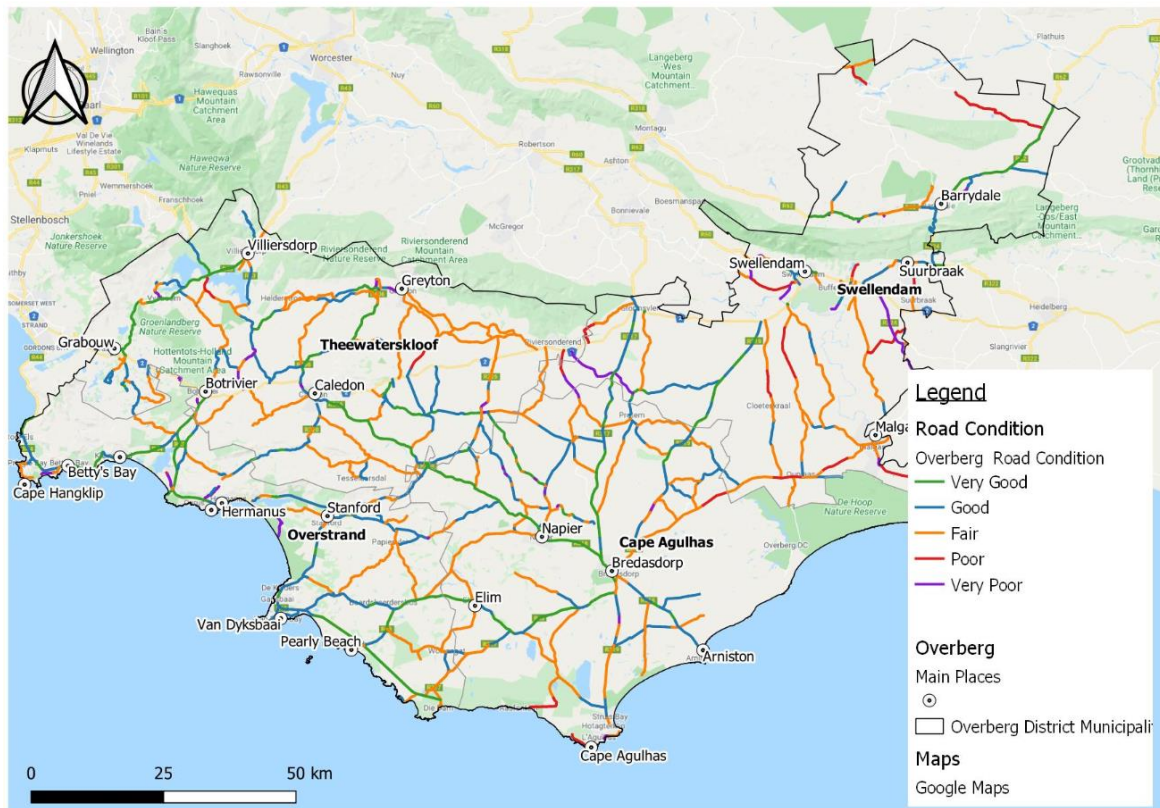
Figure 45: Overberg District Municipality road network condition
